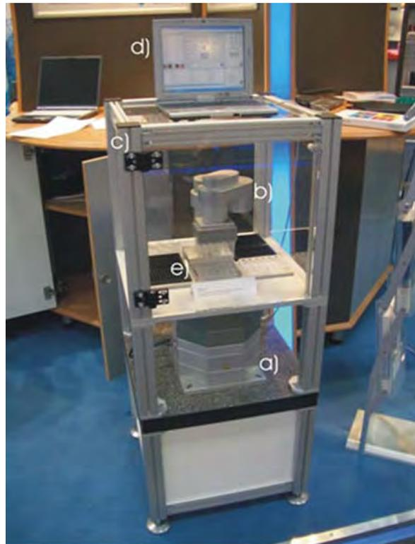
**Fig. 4.** Automated screening setup with a) Till Photonics „iMIC“ microscope, b) liquid handling robot, c) climate control chamber, d) control computer, and e) multi-well sensor plate
