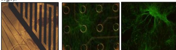
**Fig. 5.** Stem cell derived neurons overgrowing the chip surface. Left: IDES. Center: MEA electrodes. Right: Si3N4-surface.
