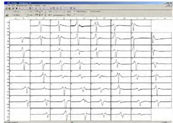
**Fig. 1:** Multielectrode array (MEA) recording of a field potential in a HL-1 cell culture. Each window represents the signal from a single electrode.
