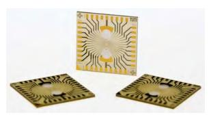
Fig. 2. Glass sensor chip without culture vessel
