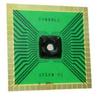
Fig. 3. Photograph of a MEA package (a glass chamber is attached in a subsequent step)
