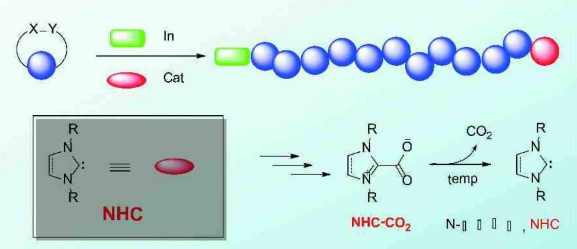
A general N-Heterocyclic Carbene (NHC) CO<sub>2</sub> adducts catalyzed ring-opening polymerization (ROP) of cyclic monomers were developed. WO2010022683
