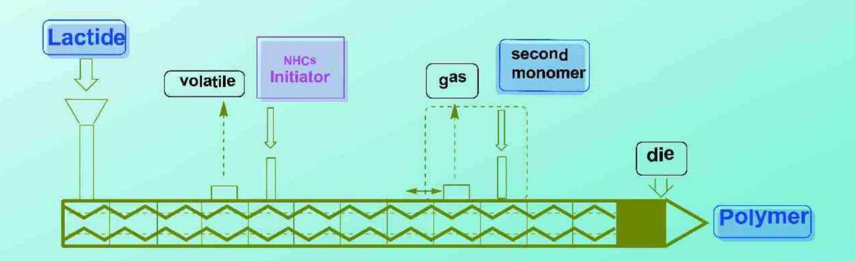
An Integrated 1-Stage Process for PLA by ROP via Reactive Extrusion
