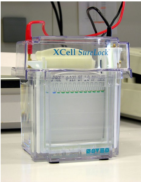
Modern gel electrophoresis apparatus in a vertical tank.
