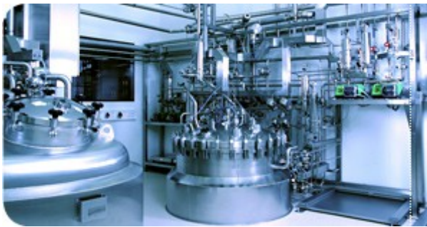
Bioreactor for the cultivation of mammalian cells used for the production of biopharmaceuticals. © Rentschler Biotechnologie
