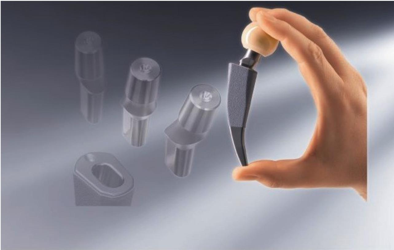
The cement-free Metha® Short Hip Stem prosthesis with Plasmapore®  $\mu$ -CaP coating of the entire proximal surface supports rapid secondary fixation.  $\mu$ -CaP is applied on the microporous titanium Plasmapore® surface. It has an osteoconductive effect and accelerates contact between the bone and the prosthesis stem.
