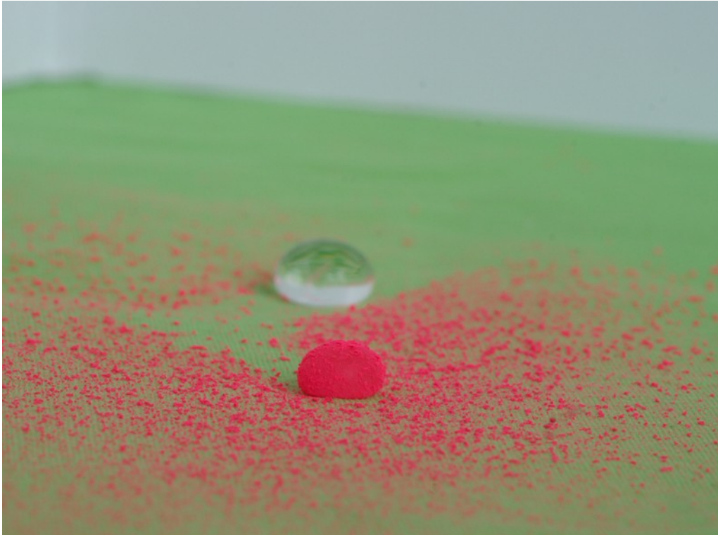
Textiles with lotus effect developed at the ITV Denkendorf © BIOPRO
