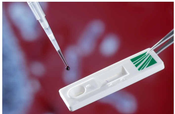
The first prototype of the pyrogen test measures approximately two centimetres by six centimetres. © Fraunhofer IGB
