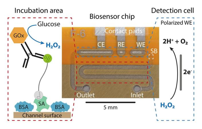
The microfluidic CRISPR biosensor measures a change in current when the sought-after miRNA, and hence biomarker, is detected in the patient sample.
