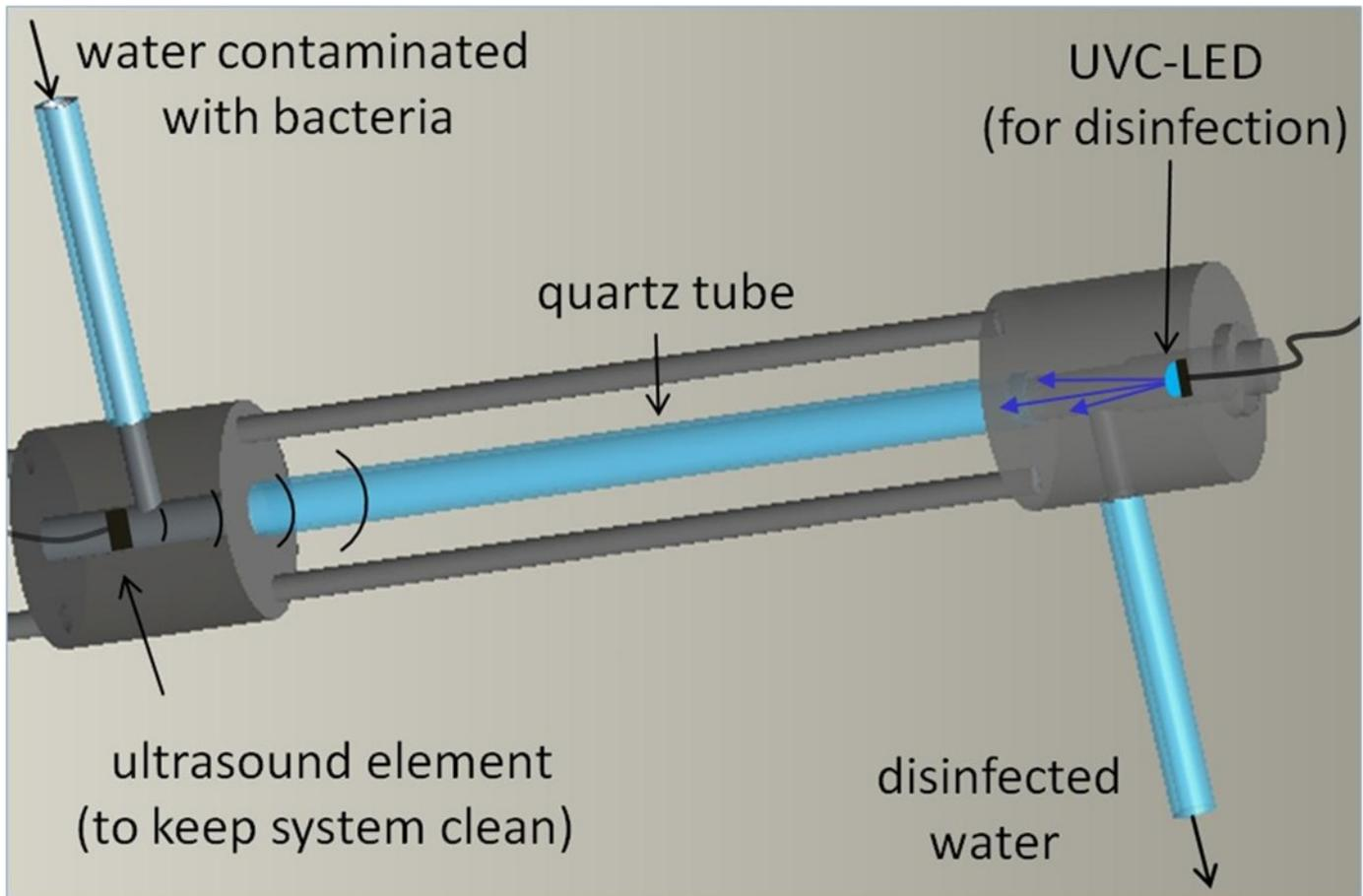
Schematic of the laboratory DNA cracker, shown here without integrated solar energy supply.
