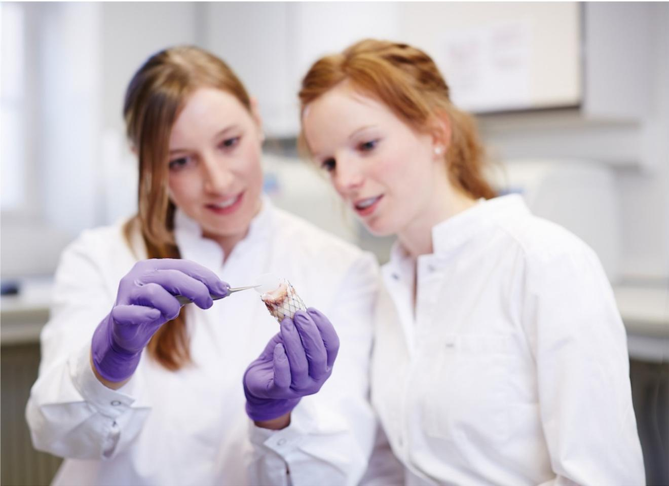
Besides the proteins that attract and bind cells, the artificial heart valve always has a synthetic component that provides stability.
