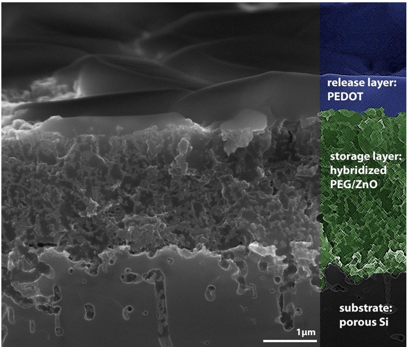
The individual layers of the drug reservoir can be discerned under a scanning electron microscope: the outer release/control layer (blue, PEDOT), below it, the storage layer consisting of hybridised PEG/ZnO (green), and all this is placed on a porous silicon (porous si) carrier layer.
