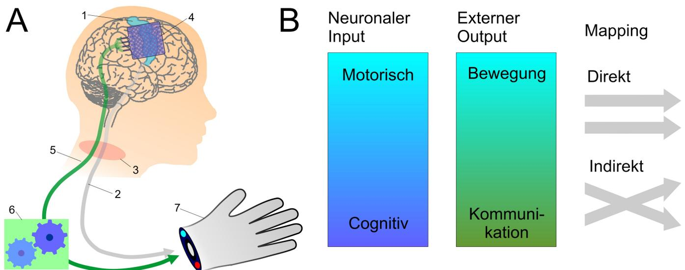
Brain-machine interface (BMI): (A) 1. Projections from the motor cortex. 2. Neurons connecting the motor cortex with the spinal marrow. 3. Lesion between brain and muscle. 4. Implanted electrode for recording motor-cortical activity. 5. Signal transmission system. 6. Determination of movement information from neural data. 7. Artificial effector system. (B) The “neural input” of a BMI can consist of a motor and a cognitive signal, which may be used to control movement or communication.
