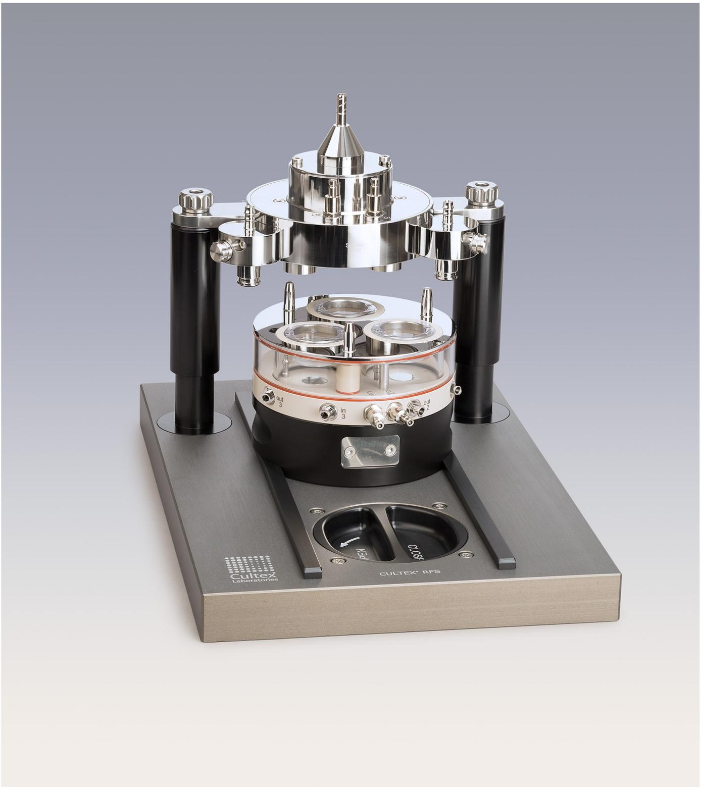
Askea Feinmechanik GmbH's cell culture reactor can be used for the in vitro analysis of air pollutants.
