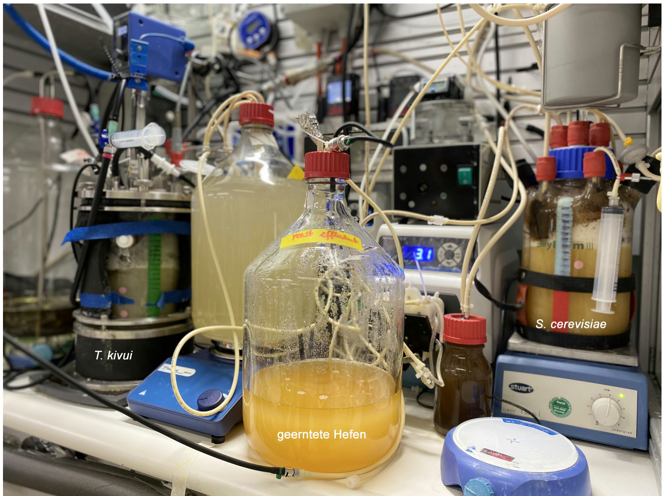
Two-stage bioreactor system on a laboratory scale. The bacterium T. kivui is cultivated in the left bioreactor and the yeast S. cerevisiae in the right. The bottle at the front contains harvested yeasts.
