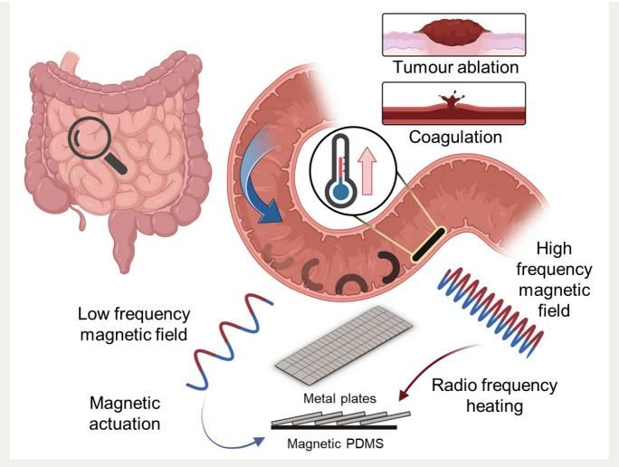
Schematic representation of how the wireless mini robot works in the small intestine. The device can be controlled using a low-frequency magnetic field; high frequencies cause the small aluminium plates to heat up, which can stop bleeding or destroy tumours, for example. Source: https://doi.org/10.1038/s41467-023-38689-x, Ren Hao Soon, CC BY 4.0 (https://creativecommons.org/licenses/by/4.0/)
