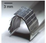
Based on the pangolin, which has armour consisting of individual overlapping hard keratin scales attached to the body, the new robot has a soft underside with a layer of overlapping, solid metal elements. This structure enables a high degree of flexibility. Source: https://doi.org/10.1038/s41467-023-38689-x, Ren Hao Soon, CC BY 4.0 (https://creativecommons.org/licenses/by/4.0/)
