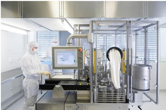
The filling system of CureVac's GMP facility conforms to the highest cleanroom standards (grade A).
