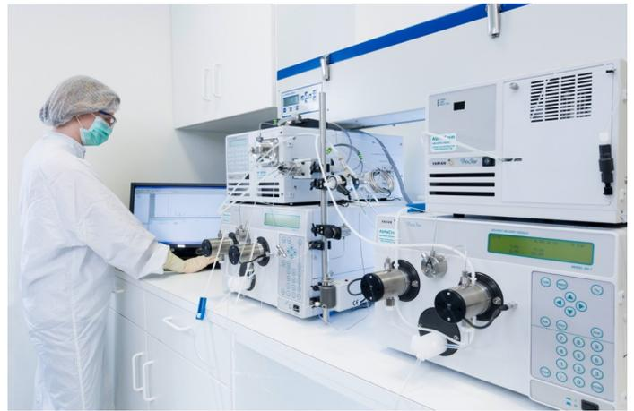
Typical CureVac laboratory with an HPLC system that is used for RNA purification.
