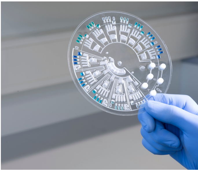
The skin sample is analysed fully automatically in a microfluidic plastic disk. © Dermagnostix GmbH
