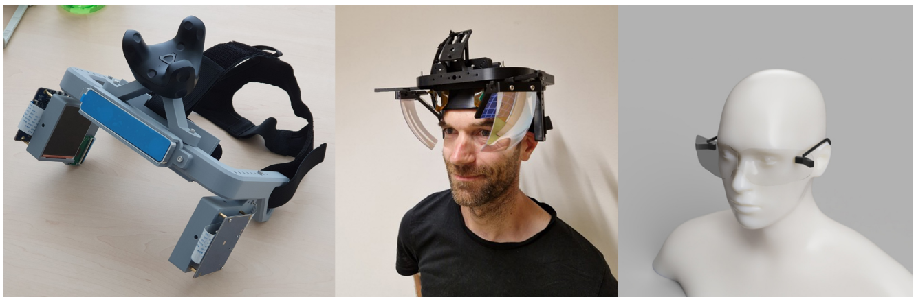
Left: First model of AR glasses with small side screens to test the preferred position of the display. Centre: Expanded model with small screens and semi-reflective lenses. Right: Future vision of AR glasses © Assländer, University of Konstanz
