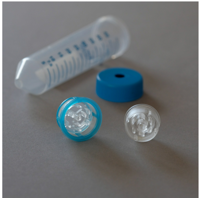
The grinder gently dissociates cells from tissue. © FFX/Dirla
