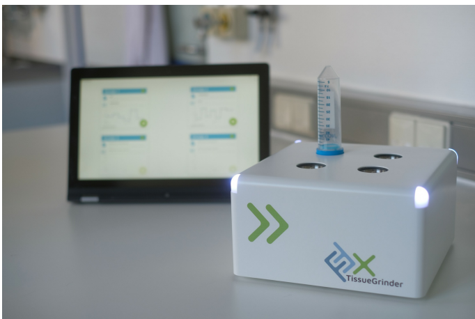
The tissue grinder consists of grinder, drive unit and control software. © FFX/Dirla
