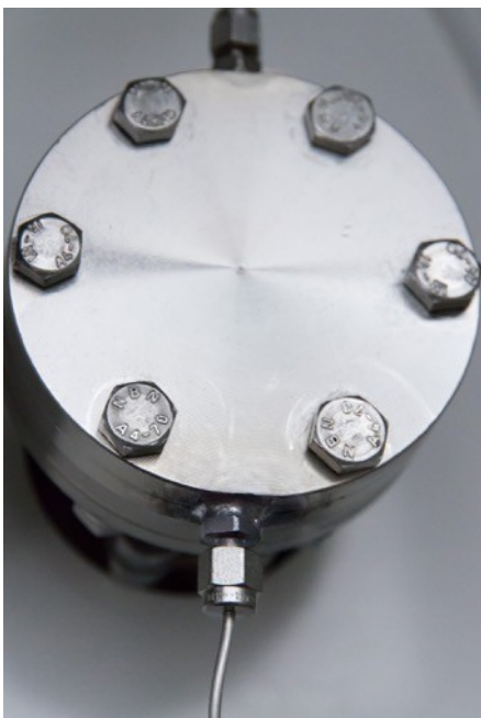
The PTFE (polytetrafluoroethylene) membrane is hidden behind the module shown. The membrane module acts as a bypass for transferring volatile compounds of a liquid into the gas phase. © Fraunhofer IGB
