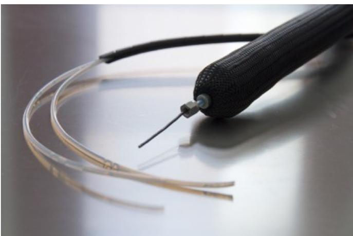
The components to be analysed are fed with the capillaries shown into the mass spectrometer through the liquid and gas inlets.
