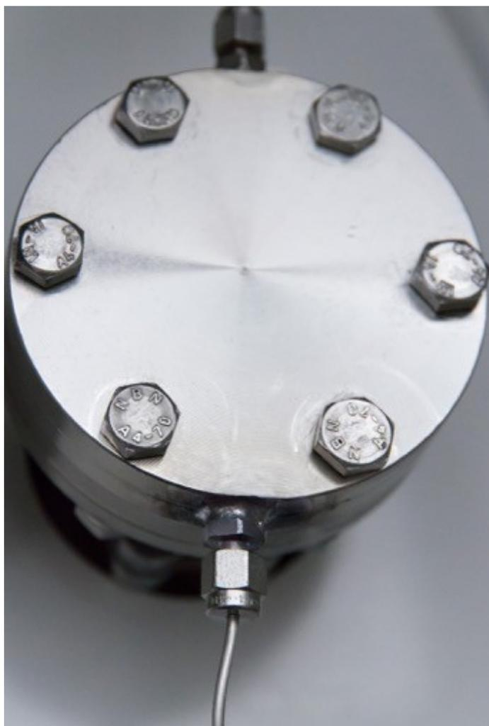
The PTFE (polytetrafluorethylene) membrane is hidden behind the module shown. The membrane module acts as a bypass for transferring volatile compounds of a liquid into the gas phase.
