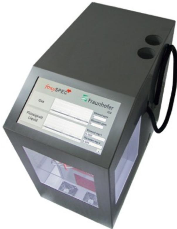
The compact mass spectrometer is about the size of a washing machine.
