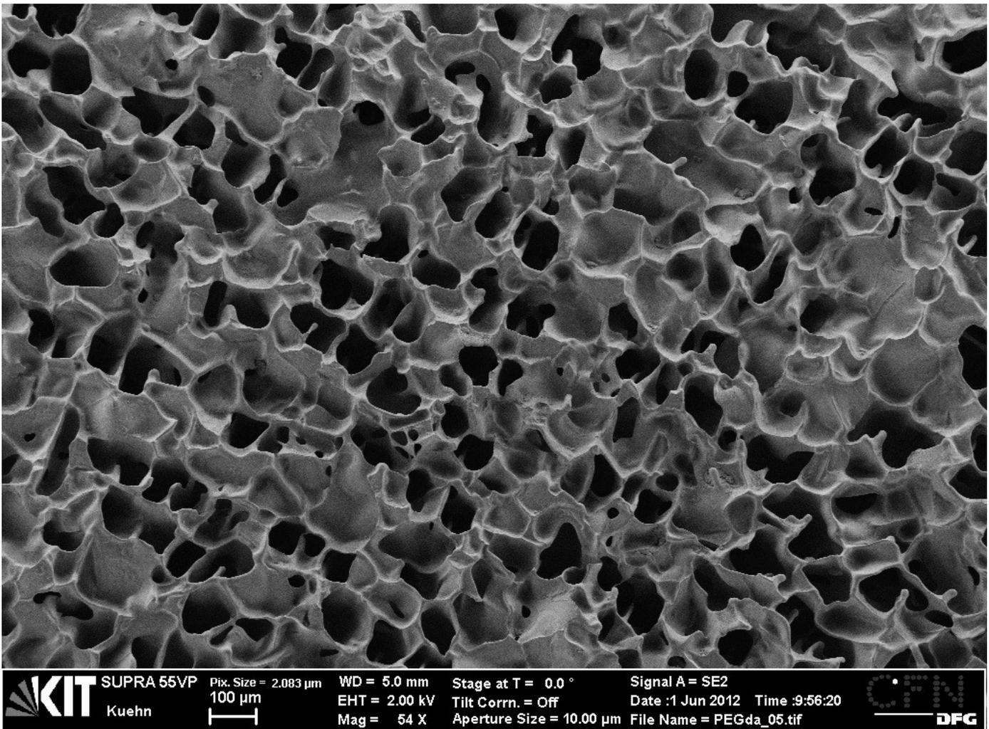
Porous, sponge-like structure of a hydrogel seen under a microscope
