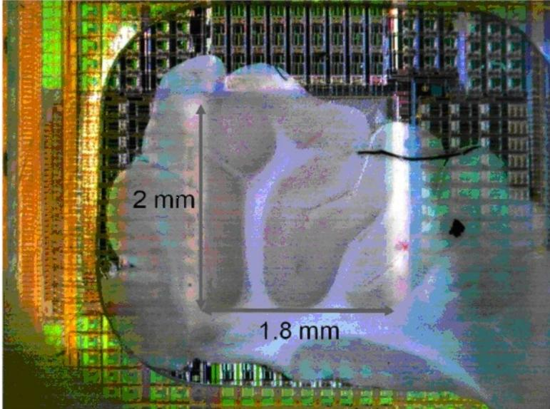
Brain slice on a CMOS-based microelectrode array (Photo: ETH Zurich)
