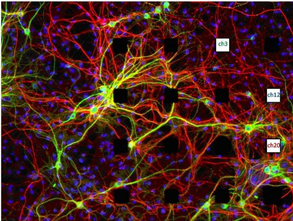
Neural network on a microelectrode array (antibody staining) (Photo: University of Hokkaido)
