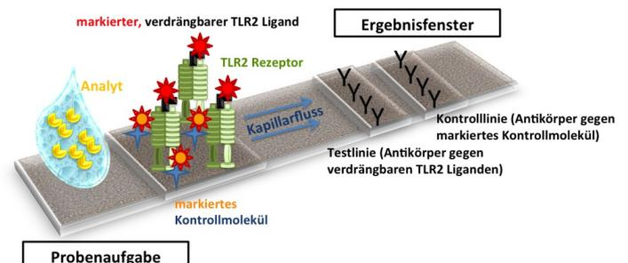
placeholders, which have a much lower receptor-binding capacity than the pyrogens. "The colour-labelled placeholders are released and migrate with the fluid through the test strip until they are visible as coloured stripes in the viewing window of the stick's result field. This colour signal shows the
