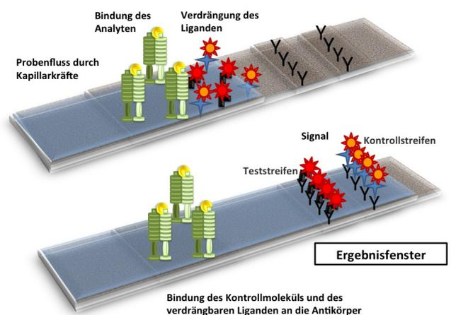
Functional principle of the ImmuStick after a sample has been applied (pyrogen is shown in yellow)
