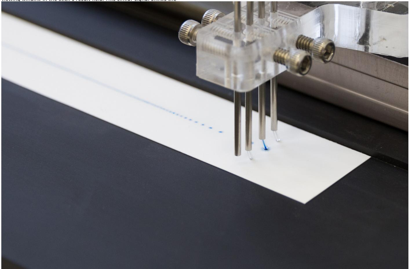
Production of the ImmuStick: application of immune receptors to the surface of the test strip.
