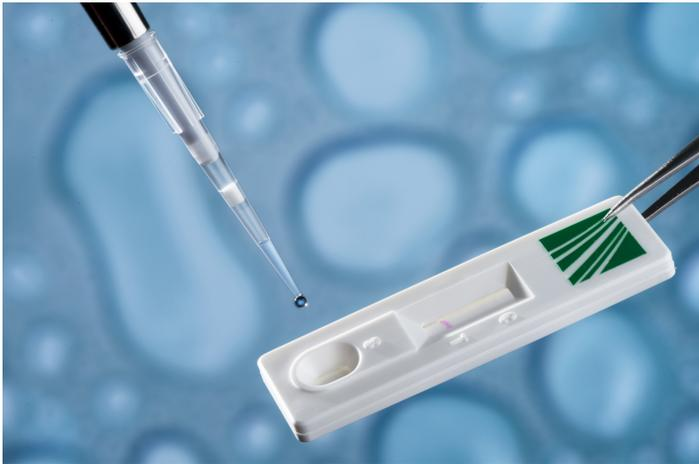
The ImmuStick can be used to identify bacteria, fungi, viruses or their pyrogenic components. The stick could potentially be used for identifying bacterial contaminations in drinking water. © Fraunhofer IGB
