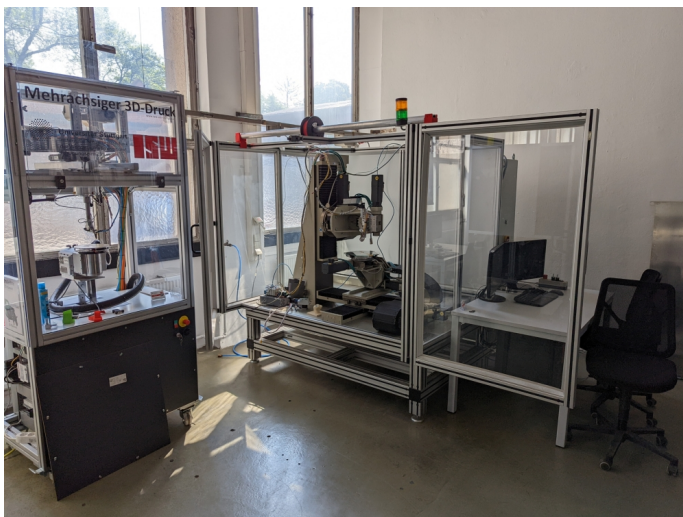
At the University of Stuttgart's Institute for Control Engineering of Machine Tools and Manufacturing Units, artificial joint cartilage is printed three-dimensionally using a novel multi-axis process. © ISW
