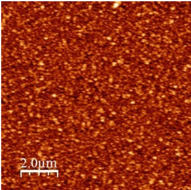
Antimicrobial surface seen under the atomic force microscope, AFM.
