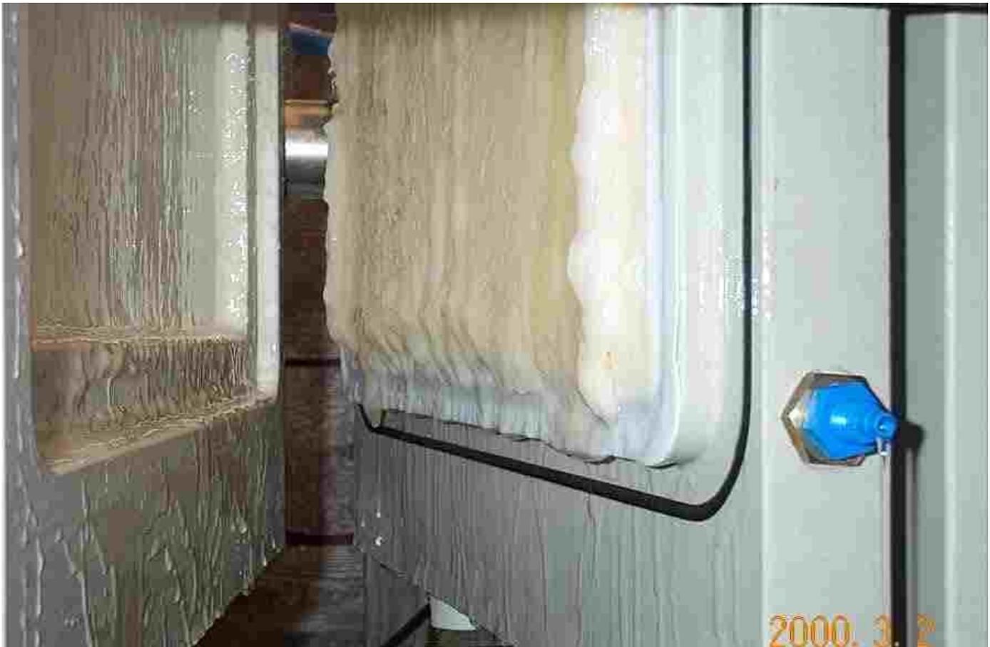
Electrofiltration of xanthane in the Symbiosis 250 pilot system: a thick xanthane layer accumulates at the anodal side of the set-up.
