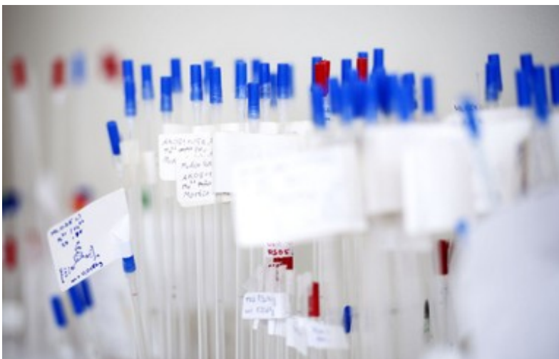
The cell suspensions used for electron spin resonance spectroscopy are transferred into special sample vials.
