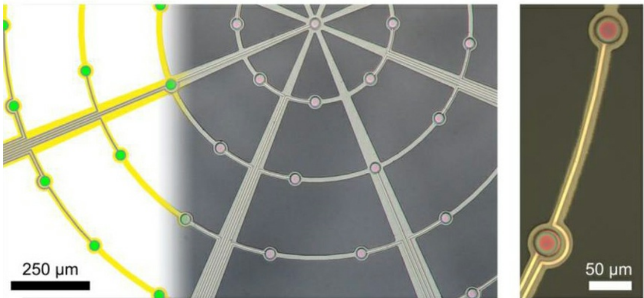
Left: The hanging spider web-like mesh with integrated microelectrodes (green) shows that the regions between the polymer filaments are open. Right: Two microelectrodes in a single filament.
