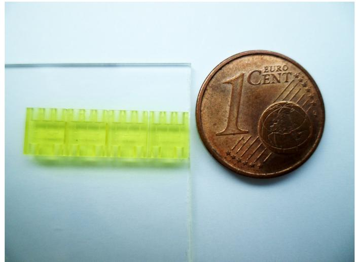
High precision manufacture of a microfluidic chip using the latest 3D printing technology. Cancer cells, drugs, reagents and oil are injected into channels less than a tenth of a millimetre in diameter to produce microscopic measuring vessels in the form of aqueous drops in an oil phase. This type of miniaturisation allows significantly more tests to be performed on patient cells than before.
