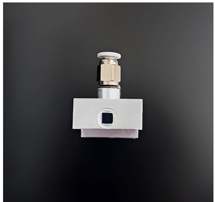
Side view of the mini-sensor with infrared-permeable barium fluoride windows, which ensure that the MIR radiation is reflected along the channel and the absorbed wavelengths of 13 CO 2 and 12 CO 2 can be measured. © Dr. Gabriela Flores Rangel/Ulm University
