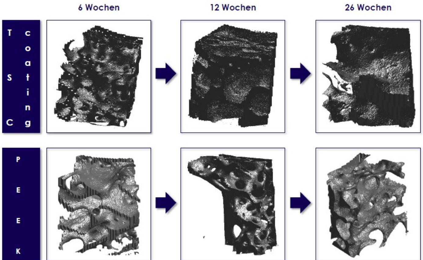
TSC combines the positive properties of PEEK and titanium – cells adhere well to the material, which also contributes to greater bone volume.
