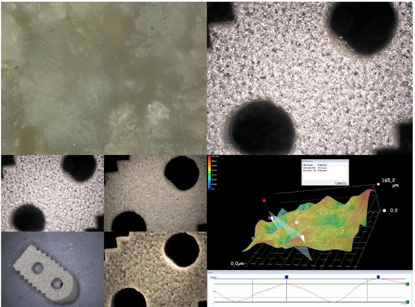
Surface topography after mechanical treatment: the texture is prepared and the surface measured before being chemically coated.
