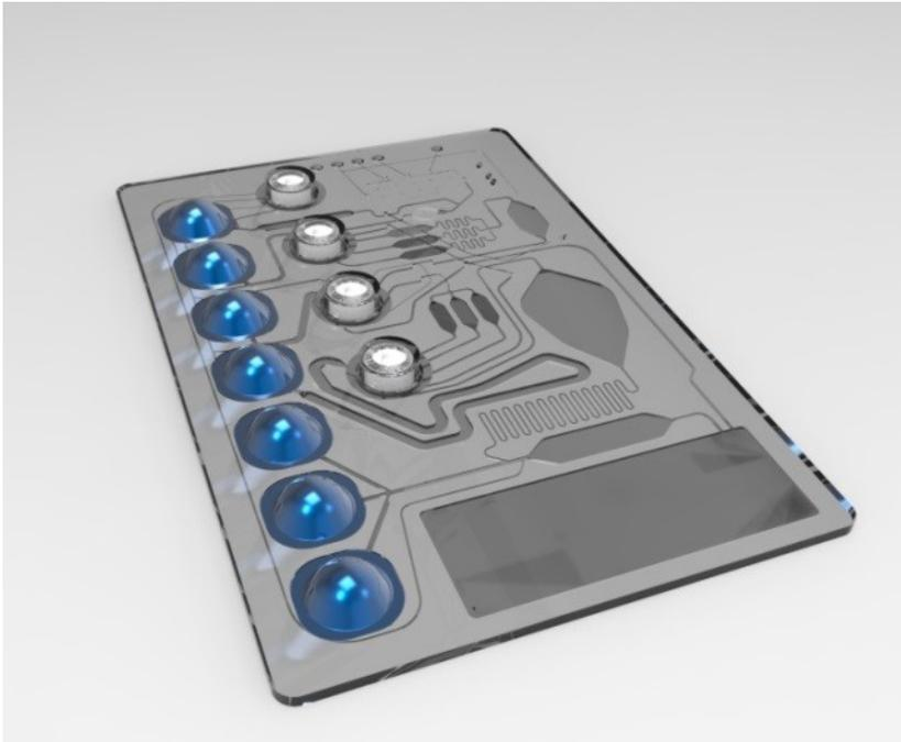
The new microfluidic chip enables automated processing of the sample and analysis of microRNAs.
