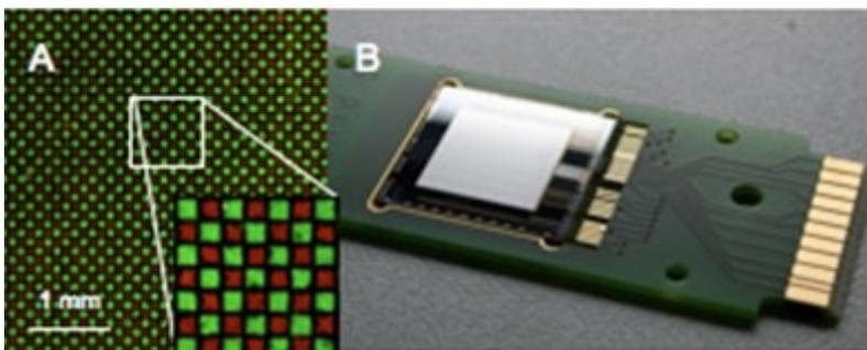
Combinatorial synthesis of a peptide array with a computer chip. Left: Pixel electrodes revealing a staining pattern caused by two different antibodies; right: plate with bonded chip.
