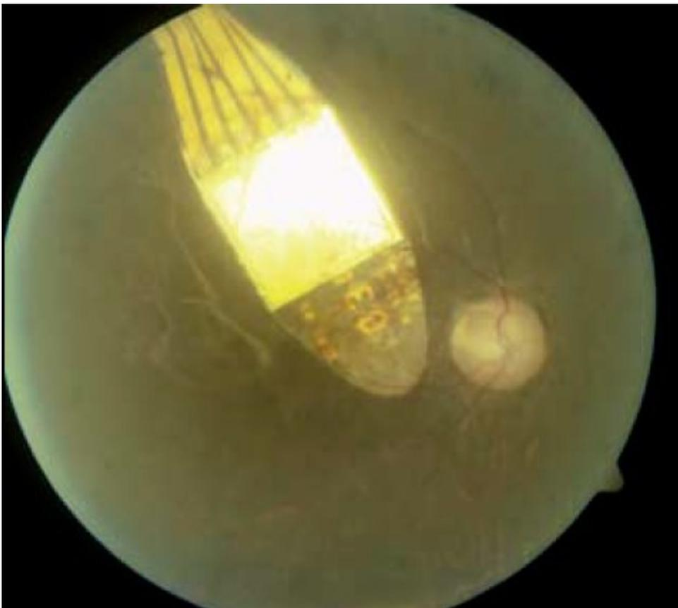
The subretinal microchip, just 3x3 mm, is placed under the retina in a spot called the macula. The chip's tiny light sensors are triggered by natural light, electrical impulses stimulate the retinal neurons in response to brightness and the optic nerve sends signals to the brain where they are translated into images.
