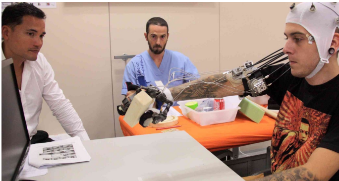
Patient testing a brain-computer interface developed at the Charité. It is used to control a hand exoskeleton.
