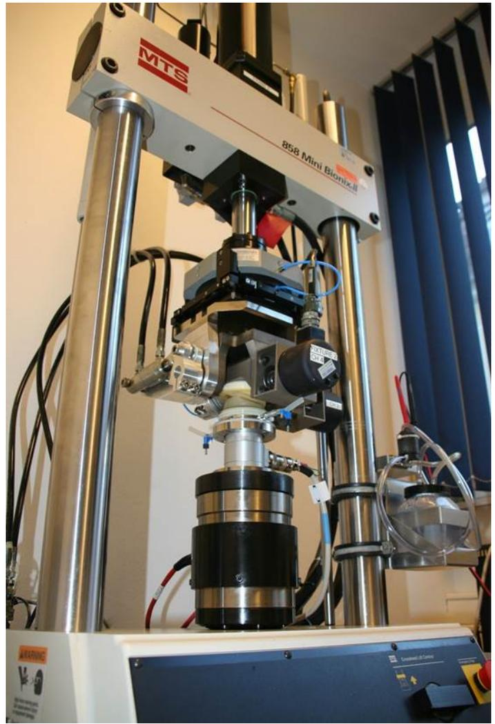
The hip simulator realistically simulates what happens with an artificial hip joint once implanted.
