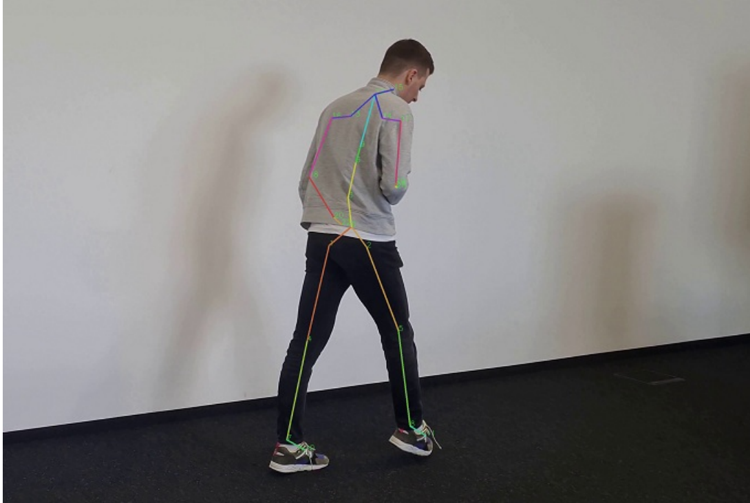
The new motion analysis system developed by the SMARTGAIT project partners enables automated acquisition of 3D skeletal data with a smartphone.
