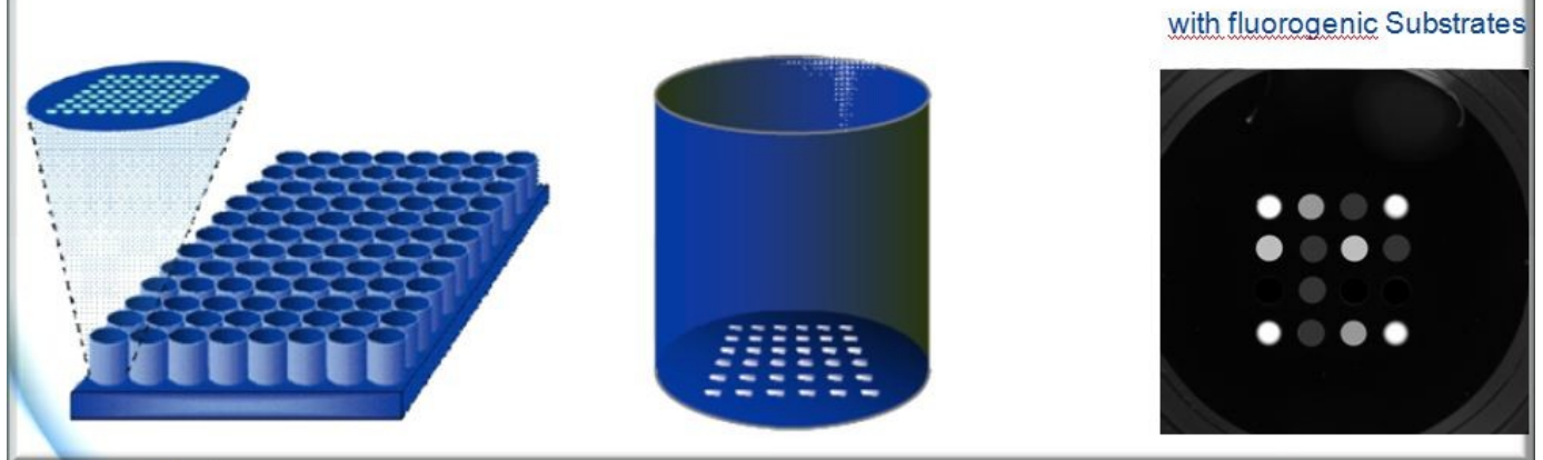
The individual wells of 96-well plate contain microarrays of 20 different allergens. © Sensovation
