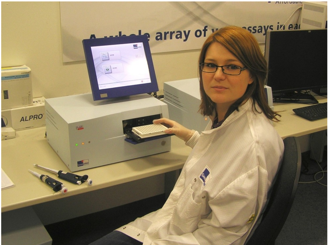
The FLAIR device enables the parallel detection of 20 allergens. © Sensovation
