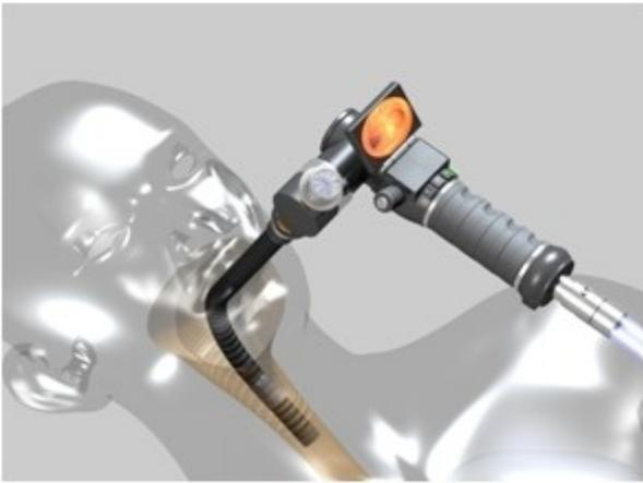
Safe and gentle: The Fibuskop® enables the examination of the respiratory tract under continuous respiration. A medical technology invention by researchers from the University Hospital in Heidelberg.
