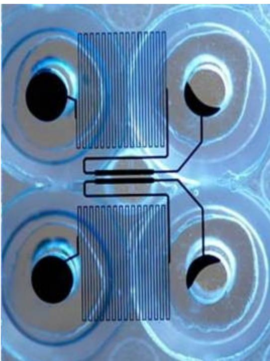
Pneumatically driven microfluidics system ("Bioflux") that enables the standardised testing of small volumes under shear flow on endothelial layers and functionalised surfaces.
