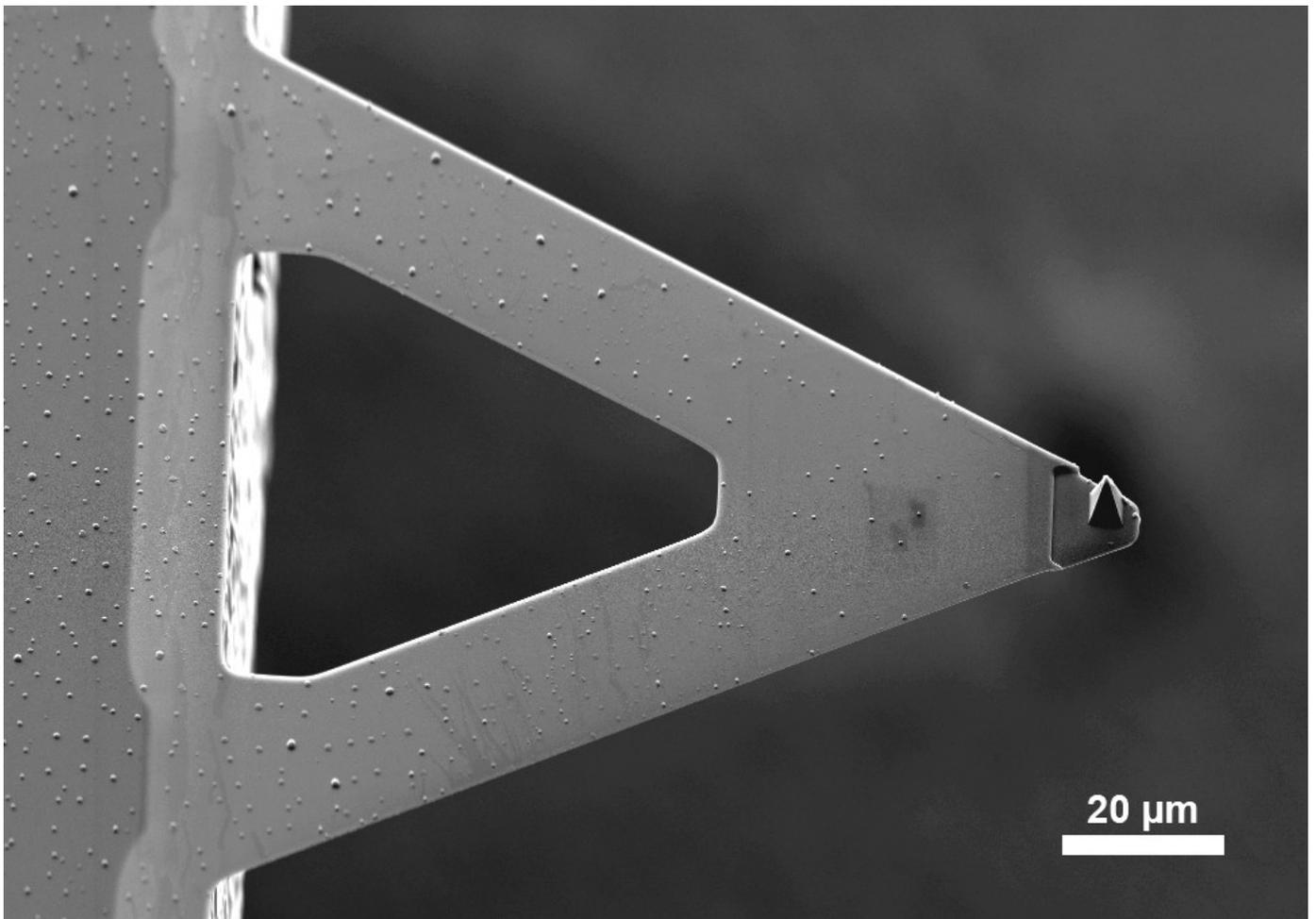
The atomic force microscope is one of Schäffer's preferred examination tools. It is equipped with mechanical probes attached to a flexible cantilever
