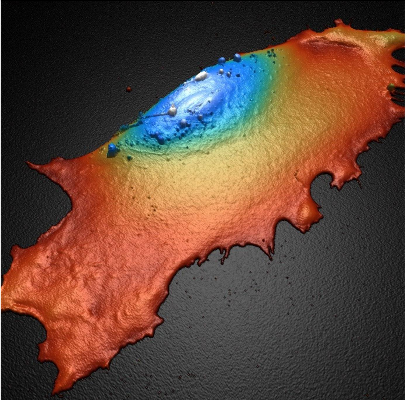
This is how cells can be represented using scanning ion conductance microscopy (SICM).
