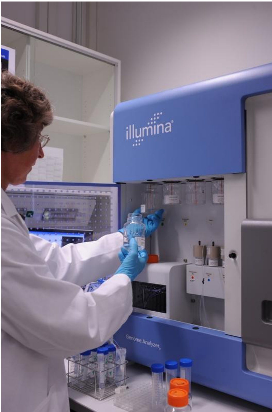
An Illumina sequencer is used to decipher the genome of Arabidopsis thaliana . © Bernd Schuller / Max Planck Institute for Developmental Biology
