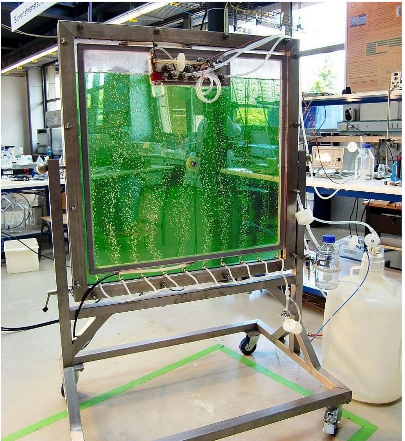
The plate reactor in the laboratory used to cultivate algae guarantees optimal light management.
