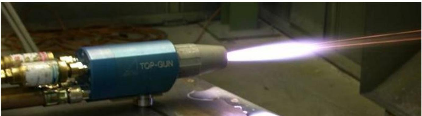
High-velocity suspension flame spraying (HVSFS) developed at the University of Stuttgart allows the use and processing of nanoscale powder materials
