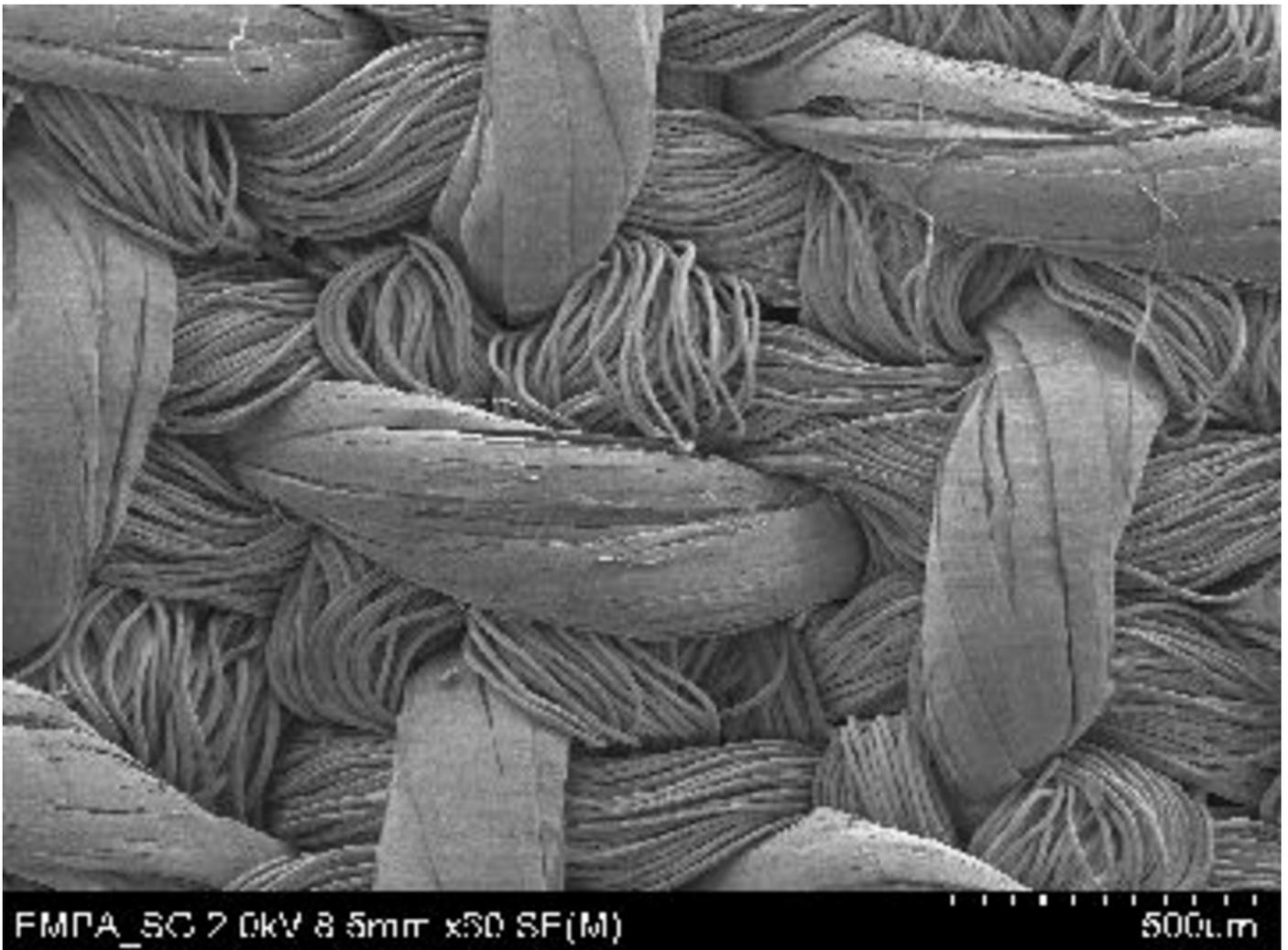
A scanning electron microscope (SEM) image of the new bed linen showing the dot-matrix like structure. The structured textile surface reduces the contact area with the skin and, thanks to the microscopic spaces between the matrix points, enables the material to absorb moisture.
