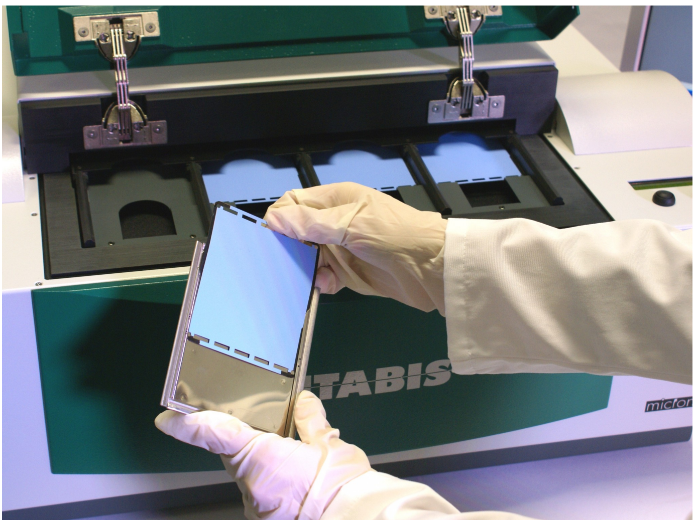
Beladen des Imaging Plate Scanners Micron © DITABIS
